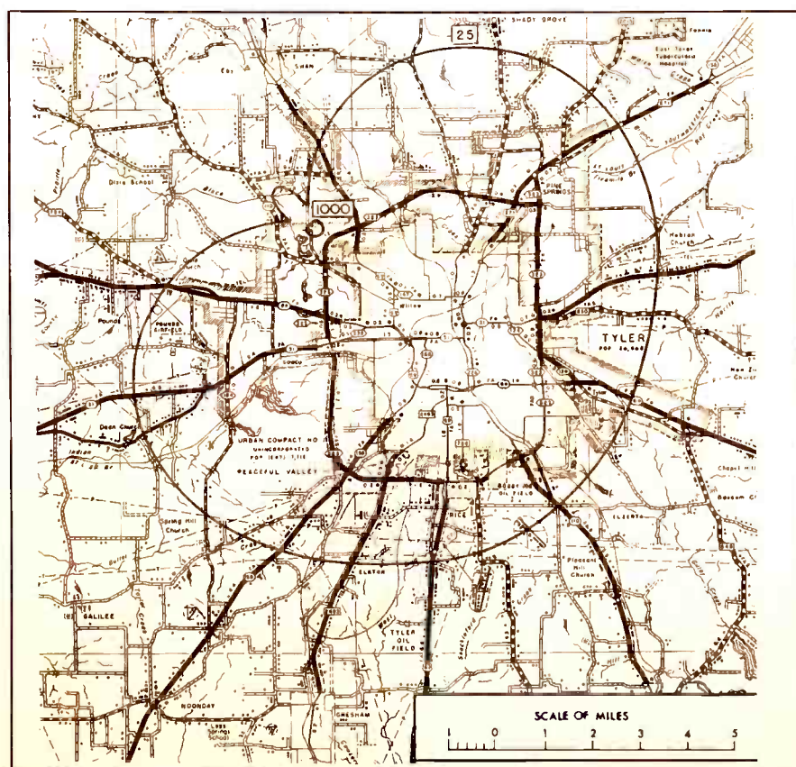
Fig. 2. Map shows 1000-, 25-mv/m contours for station whose pattern is shown in Fig. 1.
